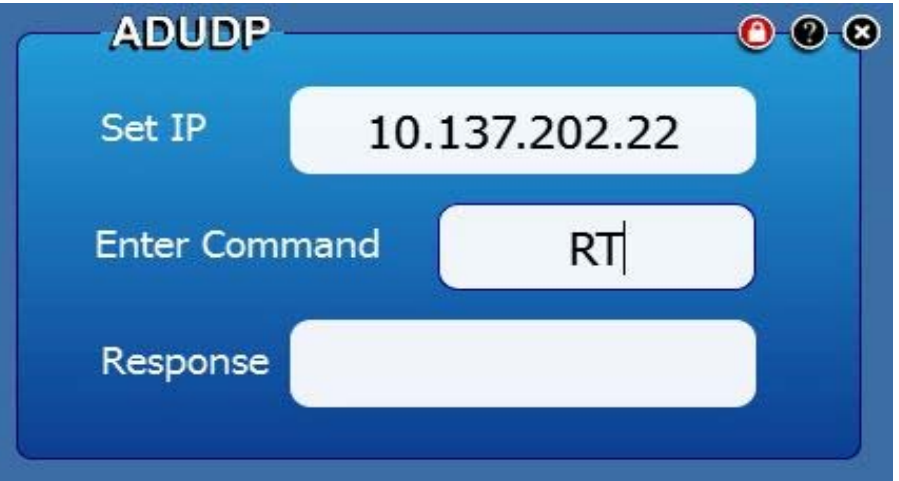
E. response from the "AD" to the "RT" command (Read Temperature)
