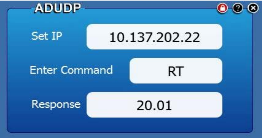
E. response from the "AD" to the "RT" command (Read Temperature)
